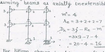
1> For beam shown in figure, find Dk. considerir eam as flexible.
