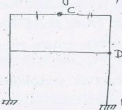
At c, one internal reaction is released.
