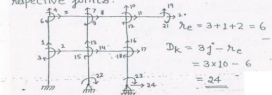
3) > For rigid jointed frame shown in figure, find Dk. assuming beams as axially inextensible.
