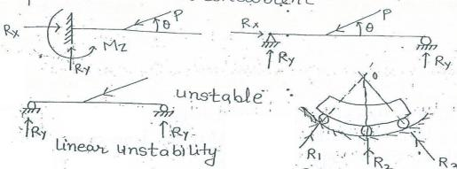
For stability of 2D structure forming three condition f static equilibrium should be satisfied.
