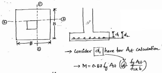
In Twoway reintorced rectangular booting slab, of in the longer direction is distributed uniformly across the bull width. In the shorter direction the total length is divided into central band of width B and edge band.
