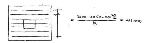
· Provide 14 no. of 20mm dia on each side at equal spacing.
