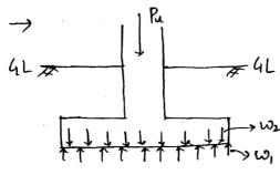
→ The slab shall be designed for Net upward - Pressure, i.e, Factored load in the Column divided by Area of booking.
