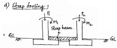
→ Strap footing controls the differential Settlement by making the two booting as a single unit and distributes the B.M., Grenerally strap beam is not designed to transfer any vertical load directly to the soil
