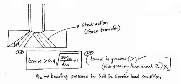
· Gross bearing Capacity; Soil load Lonsidered Gross SBC
