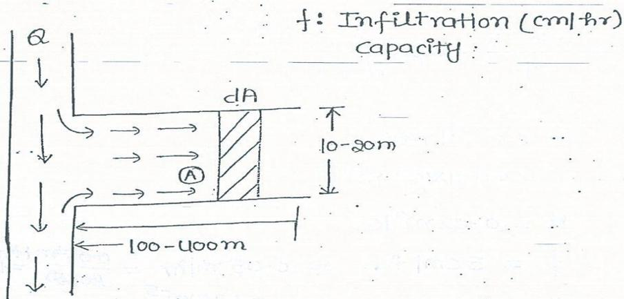
Derivation :- Time 't' required for irrigation (ing) an area 'A', for given discharge (Q).
