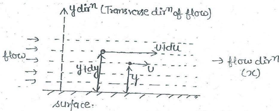
The Relative velocity of the contacting layer = zero.
