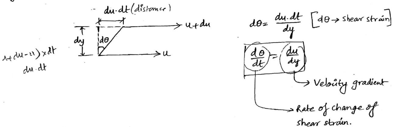
→ In case of Newtonian fluid, shear stress  $\propto$  rate of shear strain
