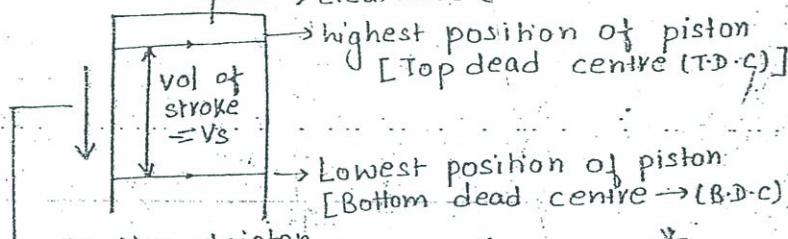
Motion of piston from TDC to BDC (stroke of piston).
