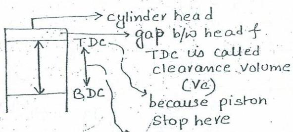
TDC is called clearance volume ( $V_c$ ) because piston stop here.
