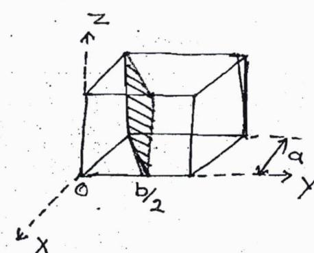
Ques:- Unit cell dimensions are  $a, b \& c$ . Determine the Miller indices for black shaded plane.
