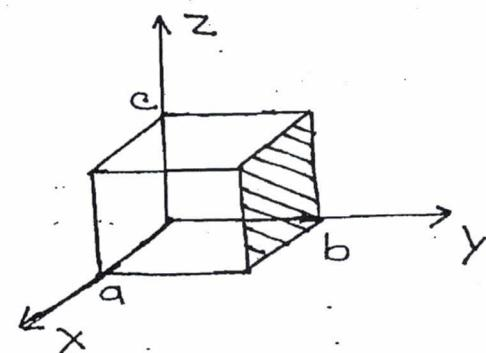
Ques:- Unit cell dimensions are  $a, b, c$ . Determine Miller indices for shaded portion
