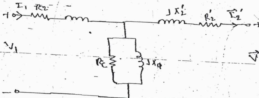
$$\begin{aligned}\vec{V}_2' &= a V_2 \angle 0^\circ \\ &= 10 \times 240 \angle 0^\circ \\ &= 2400 \angle 0^\circ \text{ Volts.}\end{aligned}$$
