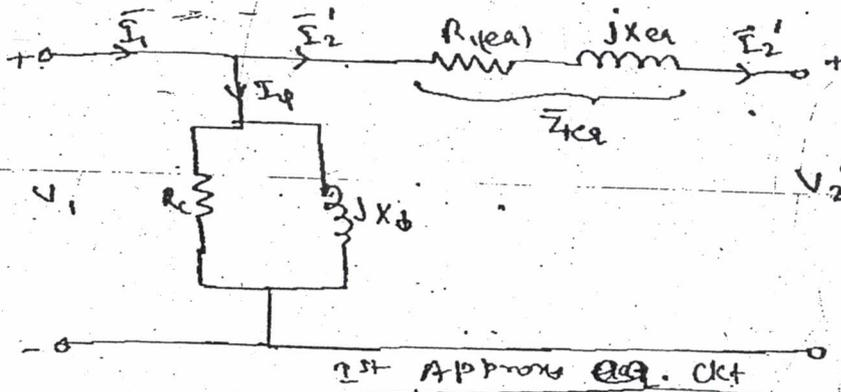
$$\vec{V}_1 = \vec{V}_2' + \vec{I}_2' \vec{Z}_{1eq} = 2453.93 \angle 0.7^\circ \text{ Volt}$$
