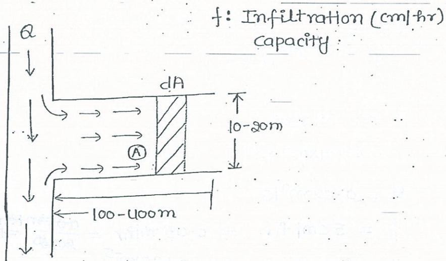
Derivation :- Time 't' required for irrigation (ing) an area 'A', for given discharge (Q).
