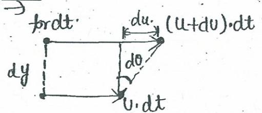
Shear deformation b/w adjacent layer =
