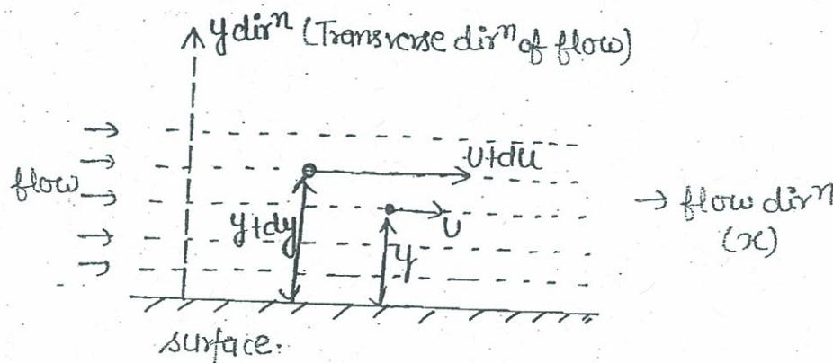
The Relative velocity of the contacting layer = zero.
