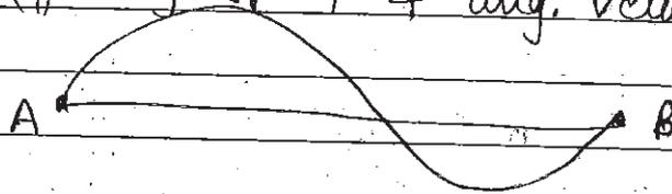
If the curve between A and B is divided by time, then we get speed, but if AB st. line is divided by time then we get avg. velocity
